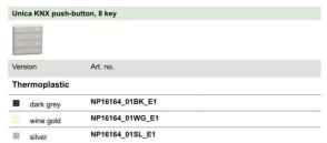
Push-button with 8 operating buttons and status indicators. In idle state, the surface of the push-button appears as a uniform plane. The inscription of the keys only becomes visible via the backlit symbols following activation. For this, you can use the enclosed prefabricated foils or the individual symbols with various motifs. Cool white and warm white LEDs show status, the brightness can be defined according to normal and night mode.
